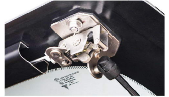
Side handle (Single handed operation) Rotary lock
